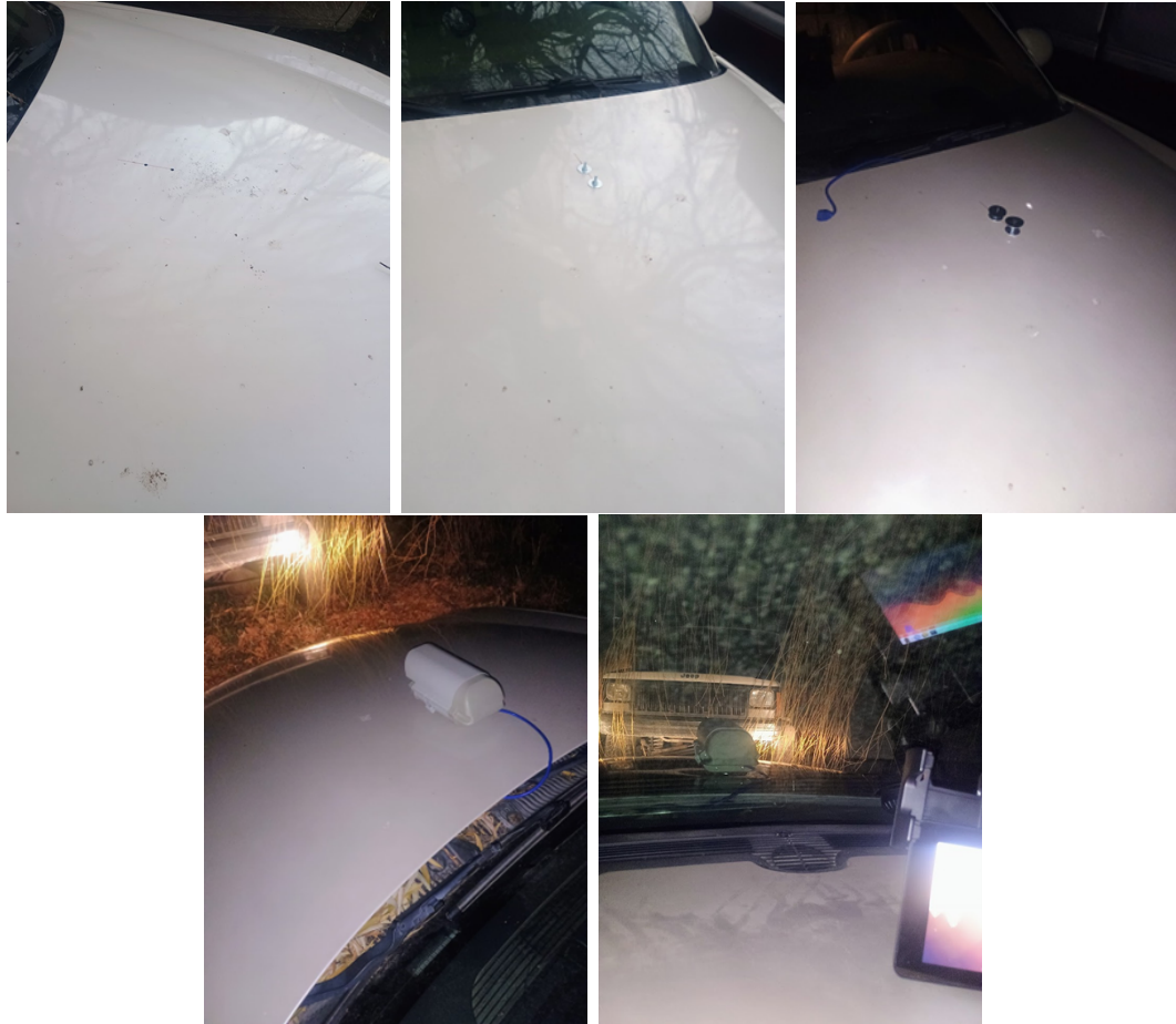
Figure 5.15 Final mounted position of the distance sensor on the vehicle. This configuration was used during experimental testing.
