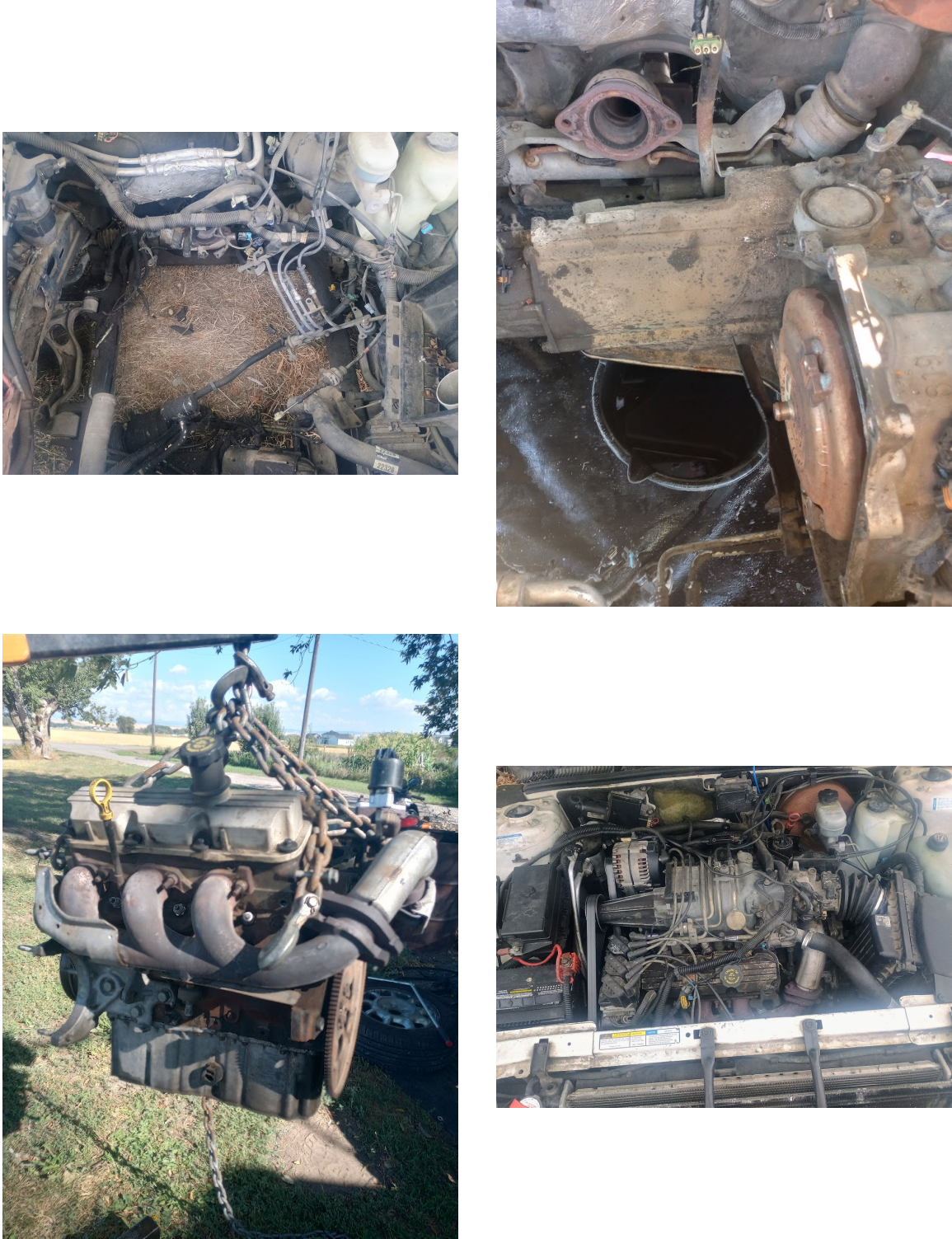
Figure 3.4 Sequence of images showing the mechanical restoration of the test vehicle, including engine and transmission removal, installation, and final assembly. This process enabled the use of a controlled and instrumented platform for experimental evaluation of the adaptive cruise control system.
