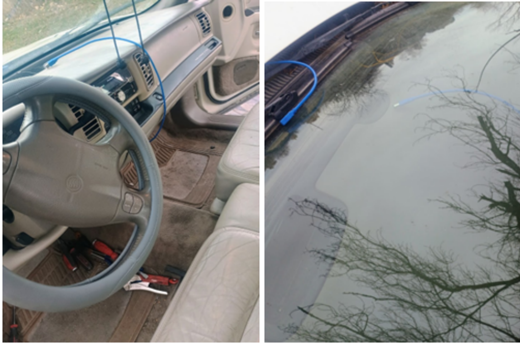
Figure 5.12 USB cable installation within the vehicle. Proper routing was necessary to ensure reliable communication and minimize interference.
