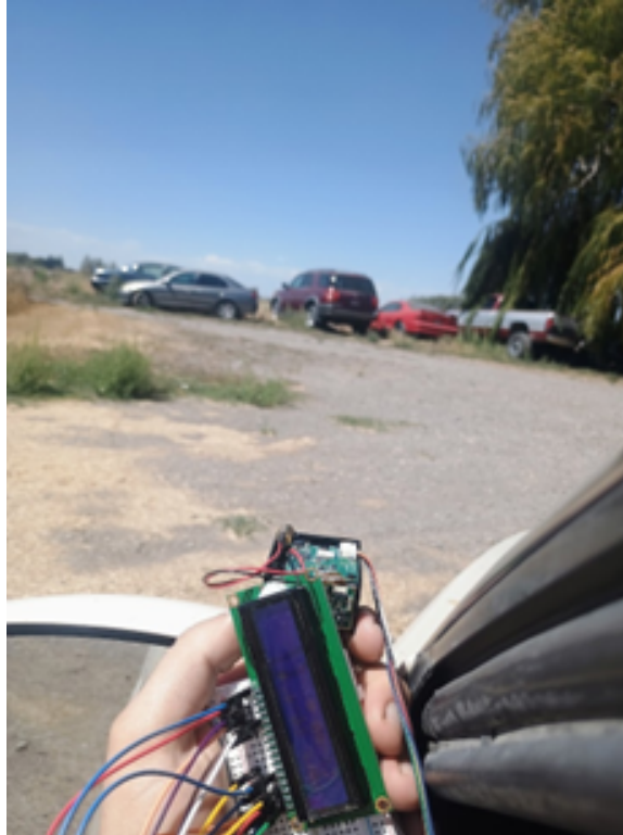
Figure 5.6 Outdoor testing configuration of the distance sensor. This setup illustrates real-world operating conditions, including environmental exposure, which influence measurement reliability.
