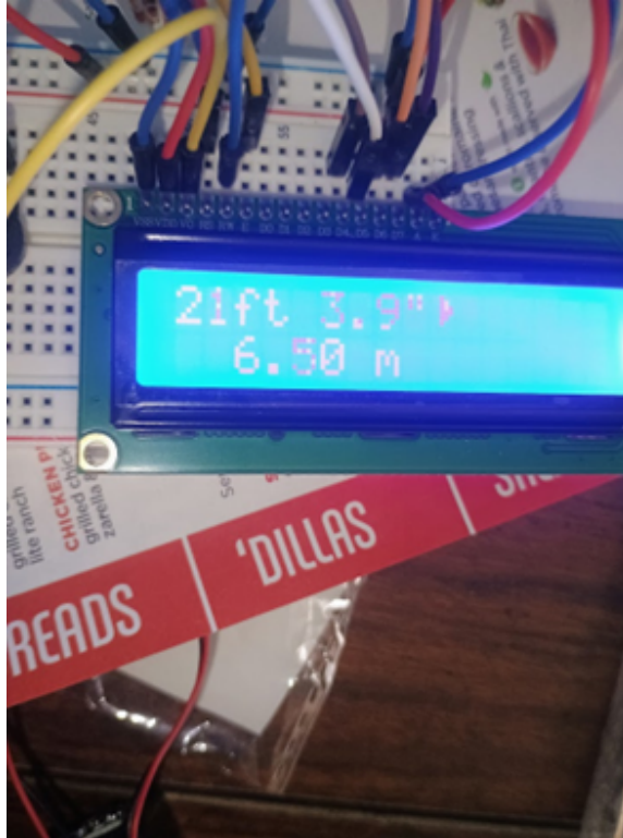
Figure 5.5 LCD displaying measured distance in real time. This visualization was used to verify correct data acquisition and communication between the sensor and processing system.
