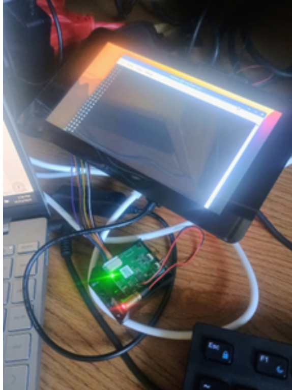
Figure 5.11 Display showing processed distance data during operation. This confirms successful integration of sensing and visualization components.
