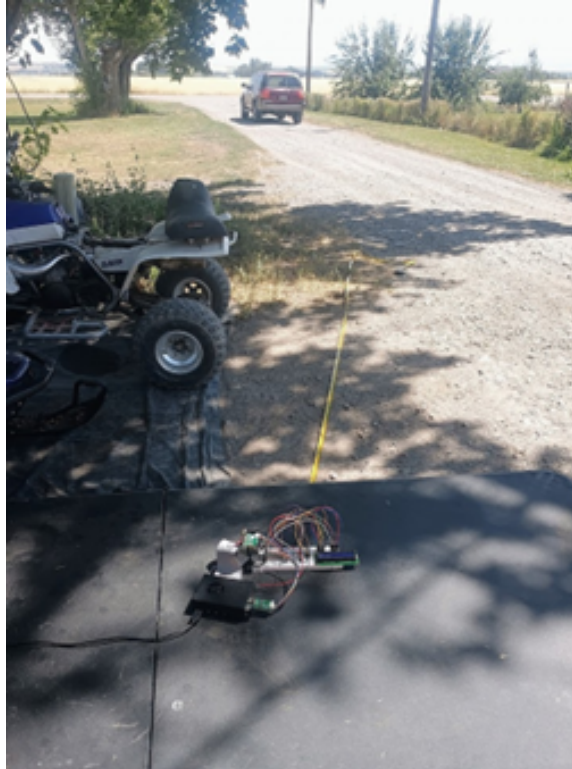
Figure 5.7 Sensor testing configuration using an external power source. This setup was used to isolate and evaluate sensor behavior independent of vehicle integration.
