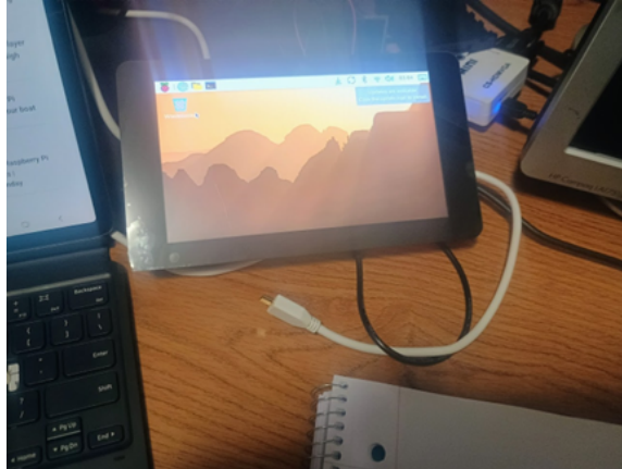
Figure 5.10 Official 7-inch Raspberry Pi display used for system monitoring. This display replaced earlier configurations and provided improved reliability.
