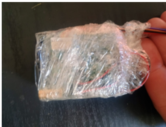
Figure 5.13 Sensor enclosure after environmental failure. Exposure to moisture compromised system functionality, demonstrating the importance of robust environmental protection.
