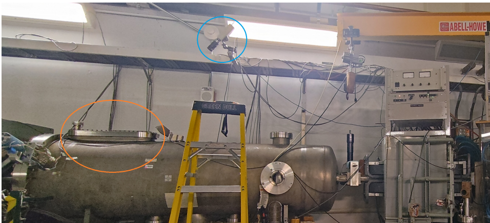
Figure 3.1 The Coffin is the large metal tank occupying the bottom left portion of this image. The blue circle is a CCTV camera that allows for remote monitoring of the beam’s path through the opening circled in orange.
