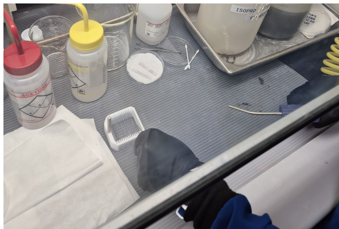
Figure 2.1 Drying the cleaned glass slides with the Nitrogen hose.
