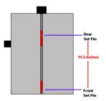
The first strip will be inserted snug up against the front channel limit pin, while the second strip will be inserted at approximately 11 inches back from the first strip. This is for a standard A4 material type size.
