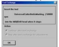
Check off the radio button labeled 'Stop after tool exchange for adjustment', and insert the tool that it is asking for. After you insert the tool, and click on 'OK', the machine will wait for you to make an adjustment.
