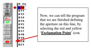
Notice that the lines of similar type, D10 through D17, are now greyed out. What this means, is that the program has recognized these apertures as being of the same type that you defined the D10 line as, and that you will not need to re-define these lines.
