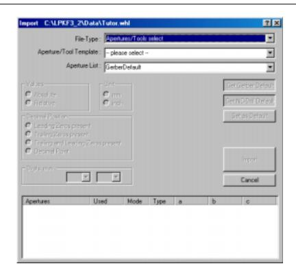
Select this file, and click on the 'open' button, to import the file. You will notice that there is no aperture information showing, and the drop down box labeled Aperture/Tool Template displays the words 'Please select'.
