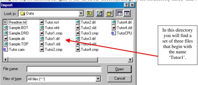
You will see that from the extensions, one is the solder side data, and another is the component side data. If you try to import either of these two files, you will notice that the aperture list information at the bottom, has question marks in it. Before you can read this type of Gerber data, you will need to import in a list of aperture information, which this file you see here, will use for it's aperture list.
