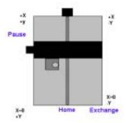
The first, is the <u>pause</u> position, where the machine head can be placed out of the way for the user to inspect and work with the tabletop. The next position to be calculated, is the <u>home</u> position, which is the central pivot point for the set pins. And the last position to be calculated, is the <u>exchange</u> position, which is where all of the tool changes will be performed.
