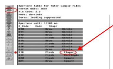
The D-code of 'D18' has a unique identifier, called 'Finger'. This aperture type, we will define as an 'Oval'. Note that on oval or rectangular shapes, you will need to define two size arguments, instead of just one.
